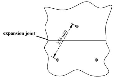
Fig. 1 . Scheme of location of the gap gauge bolts towards the expansion joint
